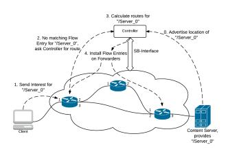
Fig. 1. SD-NDN Routing Example.
