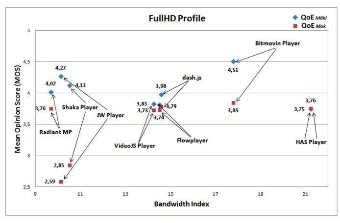
Fig. 3.  $QoE_{M\ddot{a}ki}$  (blue) and  $QoE_{Mok}$  (red) vs. Bandwidth Index for FullHD Content Profile
