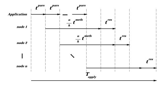
Figure 3: Time needed for a distributed operation
