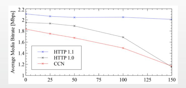
Average Media Throughput using CCN given a predefined Bandwidth Trajectory for different RTTs
