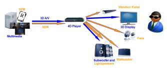
**Figure 1. Overview of Enriched 3D Multimedia Playback.** filters of the commercial Stereoscopic Player [8]. The Stereoscopic Player provides a number of different 3D modes such as side-by-side, interleaved, anaglyph, or NVIDIA 3D Vision/AMD HD3D.
