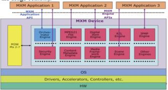
Figure 1. The MXM Architecture.
