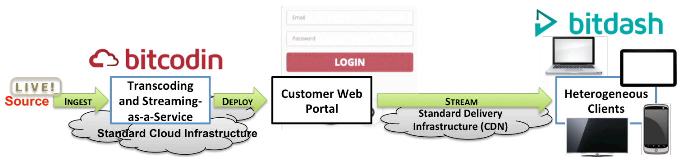
Figure 2: High-Level System Architecture for Live Transcoding and Streaming-as-a-Service.
