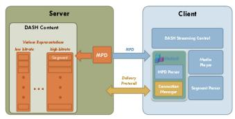
Figure 1. High-Level MPEG-DASH Architecture.
