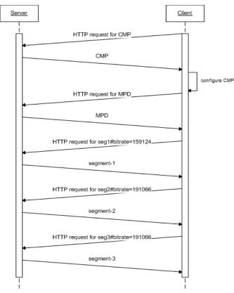
Figure 2. Sequence Diagram for CMP-enabled DASH.
